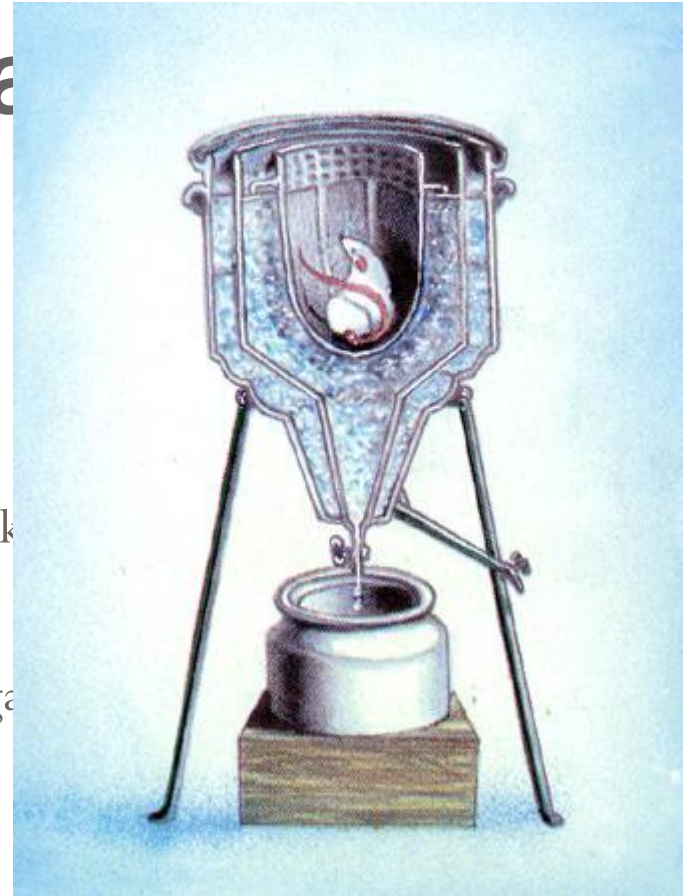
Ice calorimeter. Lavoisier and Laplace
