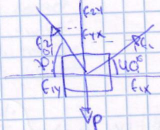
$$\begin{aligned} F_1 \rightarrow x &= \cos 40^\circ \cdot F_1 = F_1 \cdot 0'76 \\ y &= \sin 40^\circ \cdot F_1 = F_1 \cdot 0'64 \end{aligned}$$
