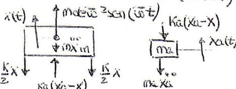
$$\begin{cases} m\ddot{x} + Kx + C\dot{x} - k_a x_a = m_d e \omega^2 \text{sen}(\omega t) \\ m_a \ddot{x}_a + k_a x_a - k_a x = 0 \end{cases}$$
