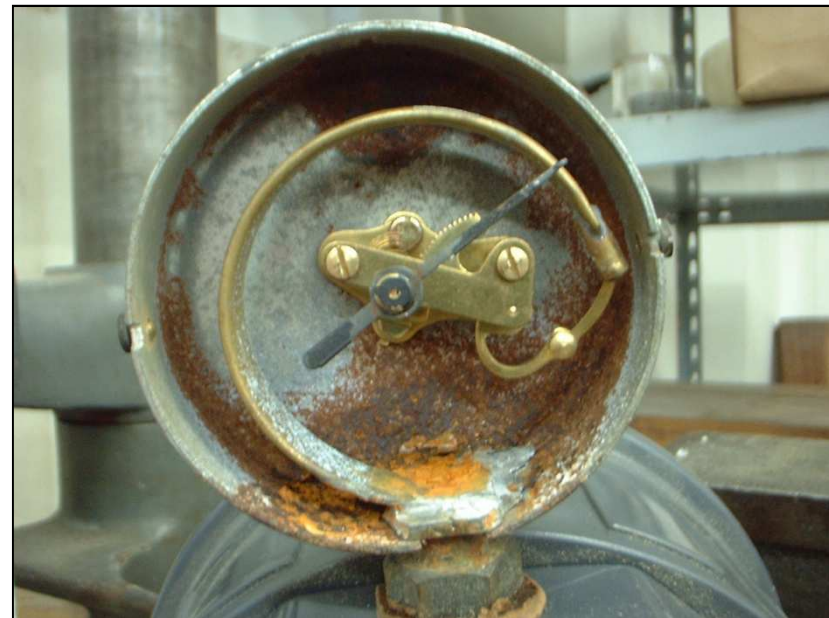
Figure 2.18 Details of the interior of a Bourdon manometer
