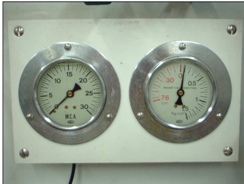
Figure 2.17 Bourdon manometer, available at the Fluid Mechanics Laboratory of the Faculty of Engineering in Bilbao. On the left hand side a typical manometer, on the right hand side manometer / vacuum meter
