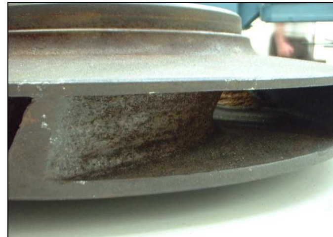
Figure 1.26. Consequence of cavitation damage on an impeller of a pump. Profile view
