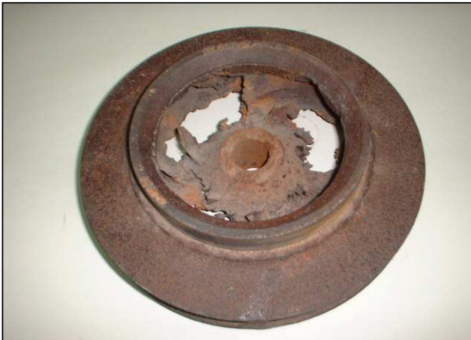
Figure 1.23. Consequence of cavitation damage on an impeller of a pump
