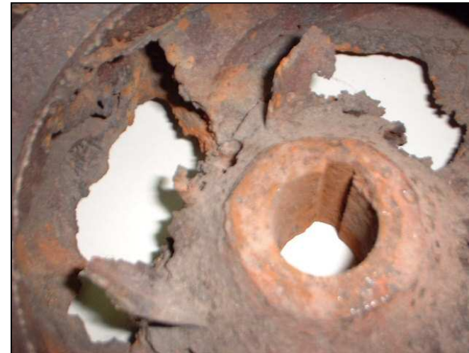
Figure 1.24. Consequence of cavitation damage on an impeller of a pump. Detail
