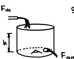
$$\frac{dV(t)}{dt} = A \frac{dh(t)}{dt} = F_{in}(t) - F_{out}(t)$$
