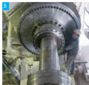
3 Alloyed steel and nitrided MT-460. 4 Torsion shaft MT coupling & special MT for paper industry. 5 & 6 Gear coupling MTG-590-HD for cement mill drive. 7 Special MTGX-420 with spacer & angular adjustment positioning. 8 Big gear coupling (o.d. > Ø 1800 mm) for steel plant converter.
