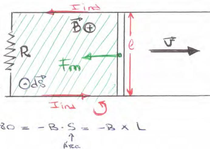
$$\Phi = \iint_S \vec{B} \cdot d\vec{S} = B \cdot \iint_S ds \cdot \cos 180^\circ = -B \cdot S = -B \times L$$
