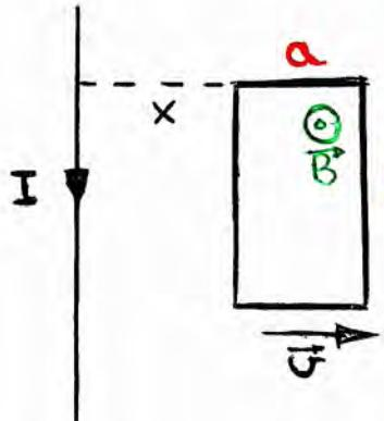
$$\Phi = \iint \vec{B} d\vec{S} = \iint \frac{x(1) + a}{x(1)} dx dy = \iint \frac{\mu_0 I}{2\pi x} \frac{b \cdot x}{ds} dx dy = \frac{\mu_0 I}{2\pi} b \cdot L \left( \frac{x+a}{x} \right)$$
