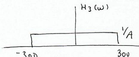
$$H_3(\omega) = \frac{1}{A} \text{LT}\left(\frac{\omega}{2 \cdot 300}\right) \rightarrow h_3(t) = \frac{1}{A} \frac{\operatorname{sen} 300t}{\pi t}$$
