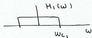
$$H_1(\omega) = \text{LT}\left(\frac{\omega}{2\omega_{c1}}\right)$$
