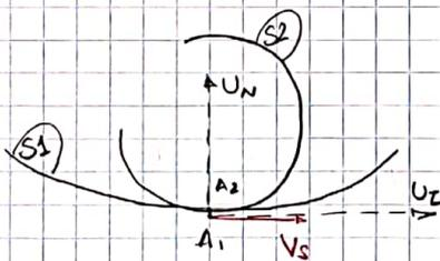
$$v_{A2} = v_{A1} \rightarrow v_{A2 \text{ n/1}} = 0$$
