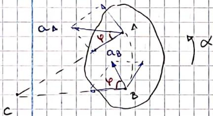
$$tg \varphi = \frac{\alpha CA}{\omega^2 CA} = \frac{\alpha}{\omega^2} = k\omega$$
