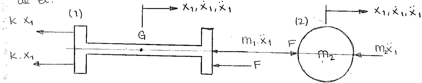
$$\begin{aligned} (1) \quad & m_1 \ddot{x}_1 + 2Kx_1 + F = 0 \\ (2) \quad & m_2 \ddot{x}_2 - F = 0 \end{aligned} \quad \left. \begin{aligned} (m_1 + m_2) \ddot{x}_1 + 2Kx_1 = 0 \\ 0.1 \ddot{x}_1 + 1000 x_1 = 0 \end{aligned} \right\}$$
