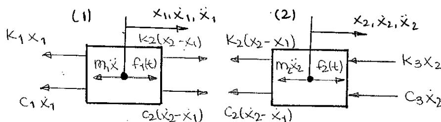
$$\begin{cases} -K_1x_1 - C_1\dot{x}_1 - m_1\ddot{x}_1 + K_2(x_2 - x_1) + C_2(\dot{x}_2 - \dot{x}_1) + f_1(t) = 0. \\ -K_2(x_2 - x_1) - C_2(\dot{x}_2 - \dot{x}_1) - m_2\ddot{x}_2 + f_2(t) - K_3x_2 - C_3\dot{x}_2 = 0. \end{cases}$$
