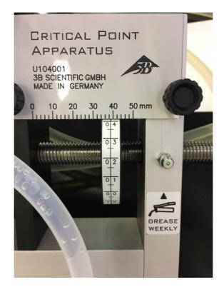
The distance measured is 38 mm + 0,4 mm= 38,4 mm
