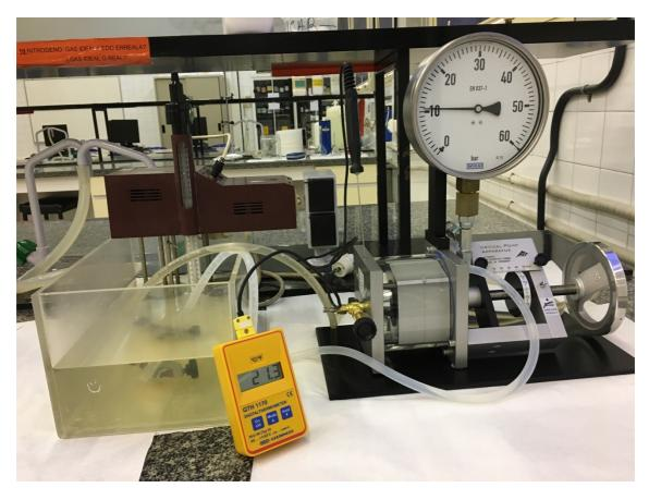
The figure also shows the flywheel used to move the piston that encloses the gas from the right. Moving the piston will change the pressure on our gas, which will be measured by a manometer (in bar) connected to the system. (1Bar =  $0.1 \text{ MPa} = 10^5 \text{ Pa} = 1/1.01325$  atmospheres).
