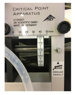
The distance measured in this picture is 40 mm + 0,0 mm= 40mm
