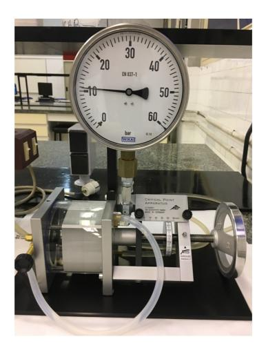
The tube is contained in a water jacket that keeps it at the **desired temperature**, as seen in the following figure on the left. Water circulates around this jacket, thanks to the motor impulse of a thermostatic bath, connected to the jacket by silicon tubes.
