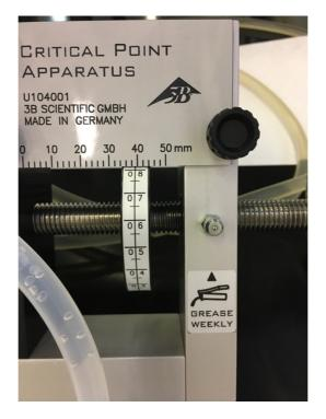
In this case, the distance measured is 38 mm + 0,8 mm= 38,8mm
